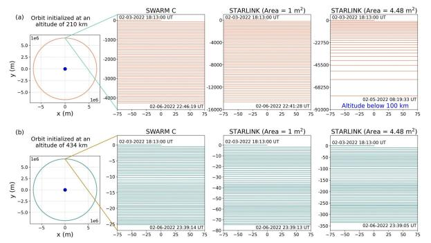
Figure 2. The plot shows simulated orbits for Swarm C and Starlink satellites with different ram areas, initialised at altitudes of 210 and 434 km respectively on 3 February 2022. The figure depicts a higher orbital decay of Starlink satellites than Swarm C under the same geomagnetic conditions.
